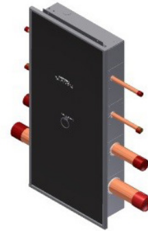
Shown above PX-VU42A2N3O4V 4 valve box with gauges ½" Medical Air, ½" Nitrous Oxide, ¾" Oxygen, 1" Medical Vacuum
